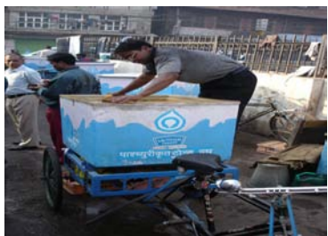
Bicycle mounted tank for distribution of pasteurized milk, Delhi.
